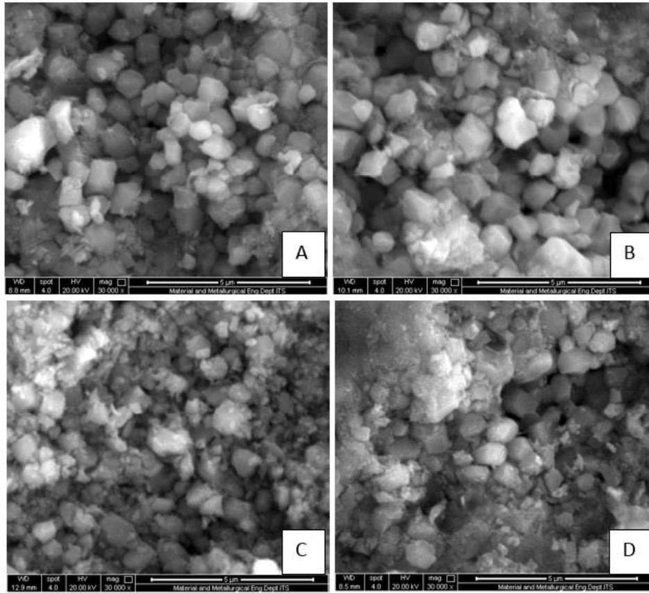
**Fig. 7.** SEM micrograph of the implants, A): F1 (BHA-chitosan = 20:80), B): F2 (BHA-chitosan= 30:70), C): F3 (BHA-chitosan = 40:60), D): F4 (BHA-chitosan = 70:30).
