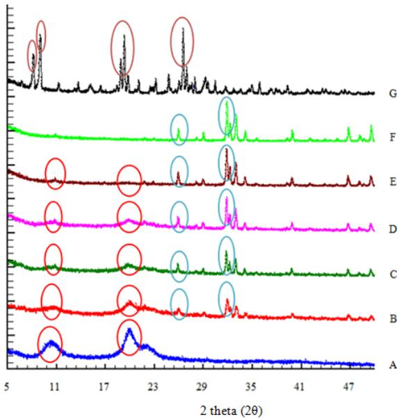
**Fig. 9.** X-ray diffraction spectrum of (A): Chitosan; (B): Formula 1; (C): Formula 2; (D): Formula 3; (E): Formula 4; (F): Bovine Hydroxyapatite; (G): Ciprofloxacin
