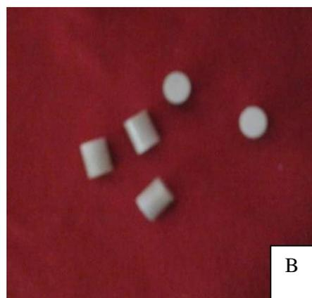
**Fig. 1.** The results of Bovine Hydroxyapatite-chitosan composite, A) slightly yellow granules, B) implants (cylindrical pellets)
