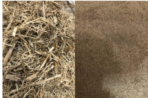
Fig. 3. Sugarcane bagasse appearance before (left) and after (right) grinding.
