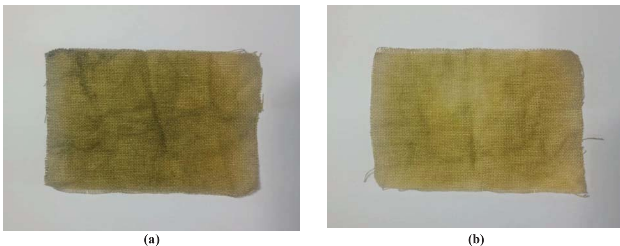
FIGURE 7. Mangifera indica Coloring Results in Linen Cloth for (a) 1:7 Ratio; (b) 1:15 Ratio
