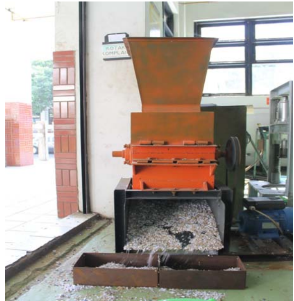
Figure 3: Diagram of the crusher by part and its physical view
