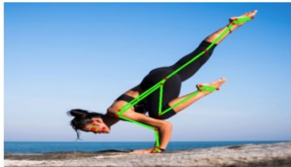
Fig. 3. The results of skeleton feature extraction using MediaPipe. Before extraction (a) and after extraction (b)
