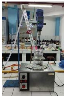
Fig. 1. Durian peel waste delignification equipment to produce natural fibers as textile raw materials
