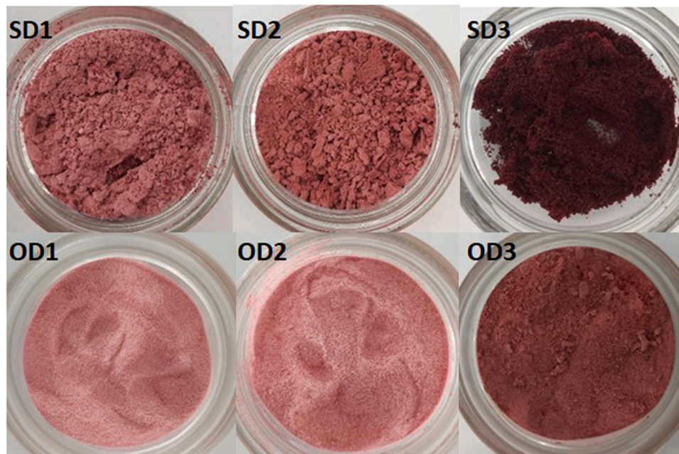
Fig. 4. Visual characteristics of roselle extract powders after spray-drying and oven-drying with various extract-to-maltodextrin ratios. Notes: SD1, SD2, and SD3 show spray-drying results with the roselle extract-to-maltodextrin (RE:MD) ratios of 1:1, 1:0.43, and 1:0.25. OD1, OD2, and OD3 show oven-drying results with RE:MD ratios of 1:20, 1:10, and 1:5.
