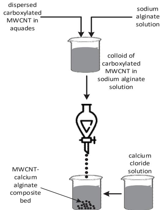
**Fig. 1.** Illustration of the process of synthesis of a composite of PWNC/ calcium alginate using the impregnation method.
