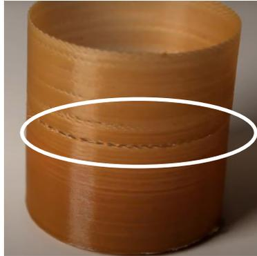
**Gambar 5.9.** *Under-extrusion*
