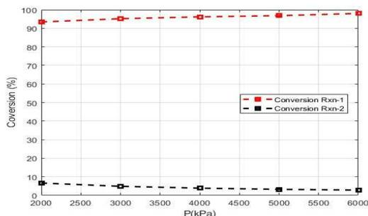
Fig. 7 Conversion vs Pressure at T=150 C
