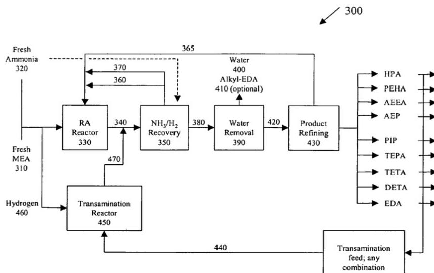
Fig. 1 Flowchart of Ethylenediamine Production, Source: [19].
