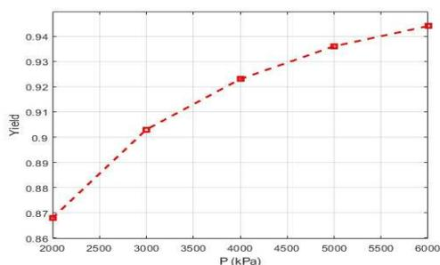
Fig. 6 Yield vs Pressure at T=150 C
