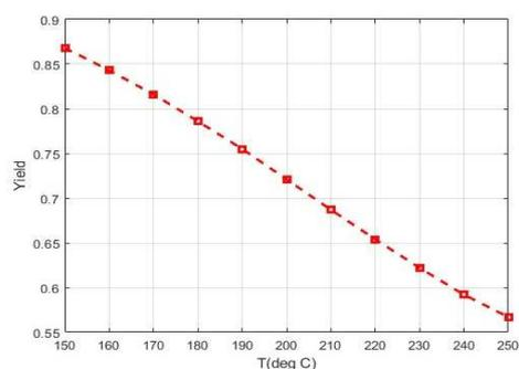
Fig. 4 Yield vs Temperature at 2000 kPa
