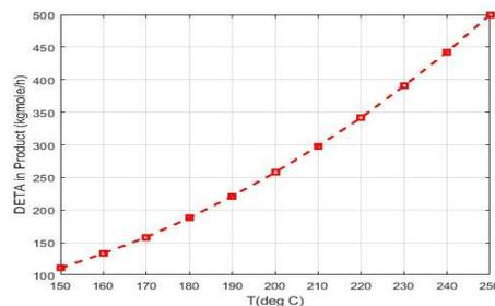
Fig. 9 DETA in Product vs T at 6000 kPa
