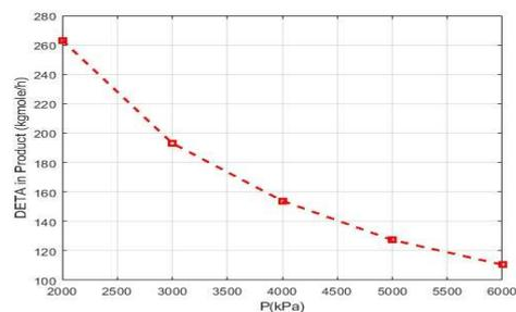
Fig. 8 DETA in Product vs P at 150 C
