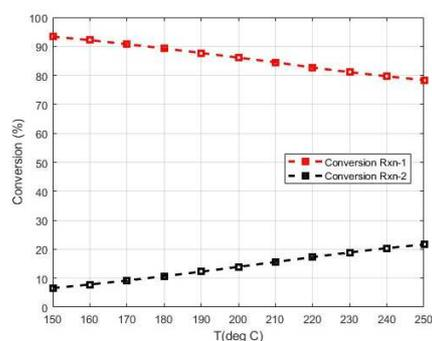
Fig. 5 Conversion vs Temperature at 2000 kPa
