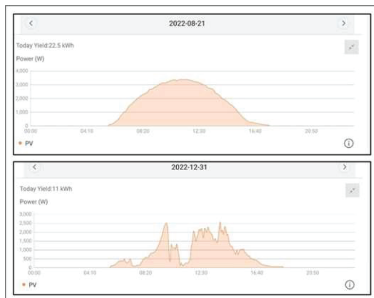
Figure 5. Diurnal power output and the total energy yield for two different weather conditions: clear day (upper), and cloudy day (lower)
