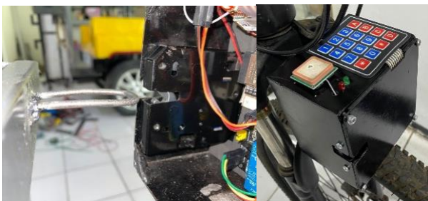
Fig. 3. The locking setup of the bicycle access and monitoring system
