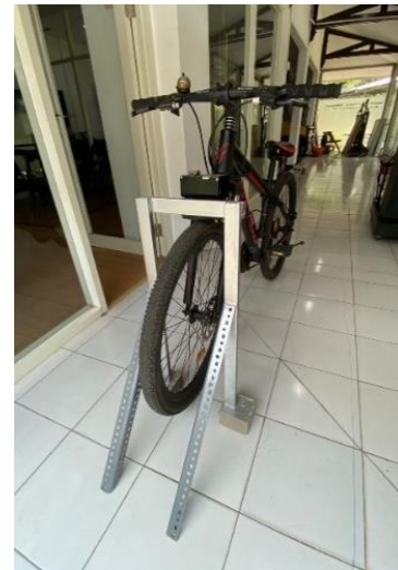
Fig. 4. The holder stand of the bicycle access and monitoring system
