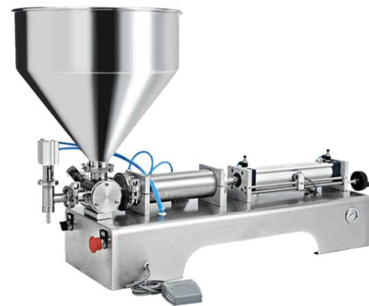
Figure 1. Semi- Automatic Pneumatic Filling Machine & Anatomy
