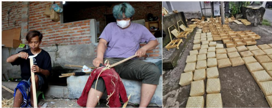
Figure 5. Bamboo processing using manual tools and solar drying
