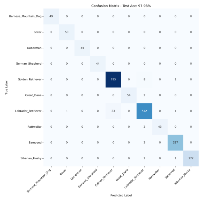
Figure 5. Confusion Matrix of the Proposed YOLOv8n–ViT-B/16 Framework Showing Classification Performance Across Ten Dog Breed Categories Using 2,133 Test Images.
