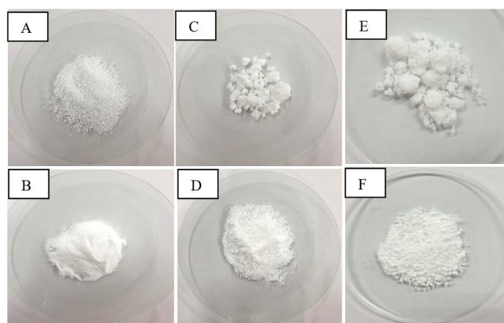
Figure 1. Visual appearance of pure materials, physical mixture, and cocrystal. (A) Citric acid, (B) Nicotinamide, (C) CN-PM 1:1, (D) CN-PM 1:2, (E) CN-Cocrystal 1:1, (F) CN-Cocrystal 1:2
