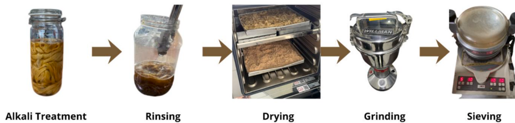
Fig. 1. Schematic representation of the fiber preparation process, including alkali treatment, rinsing, drying, grinding, and sieving.
