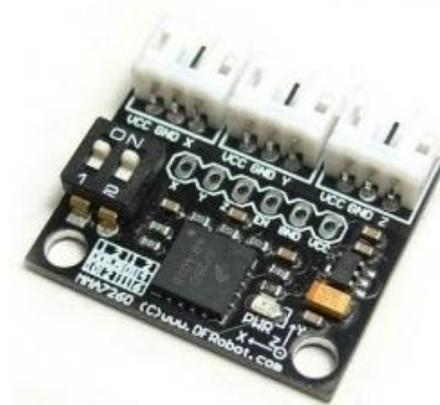
Gambar 17. Sensor Accelerometer MMA7361
