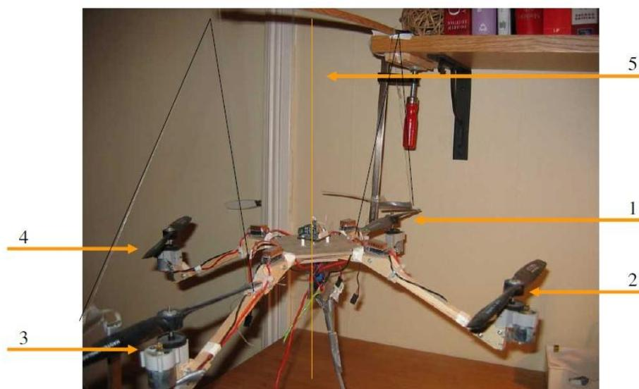
Gambar 7. Model *Quadcopter* Berbahan *Polystyrene* [3]
