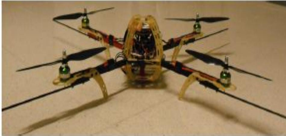
Gambar 4. *QuadCopter Prototype* [2]
