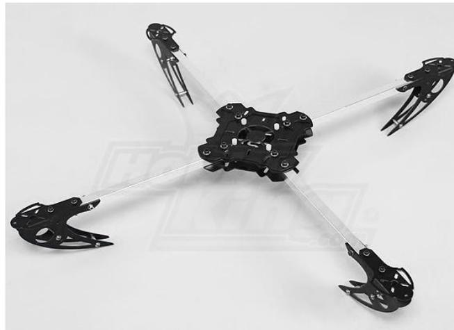
Gambar 10. X525 Glass Fiber QuadCopter Frame 60 cm [5]
