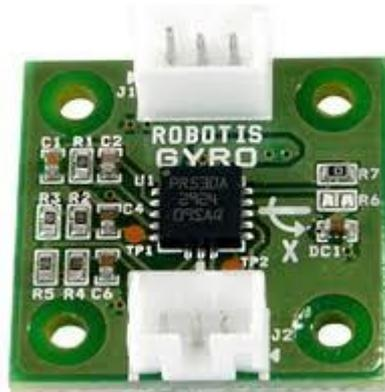
Gambar 18. Sensor Gyroscope GS-12
